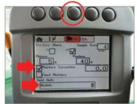
2. To make a moisture correction, roll your armrest dial to the moisture correction section. Once that is highlighted press the check mark on the arm rest. When you push the check mark the box will go black.
