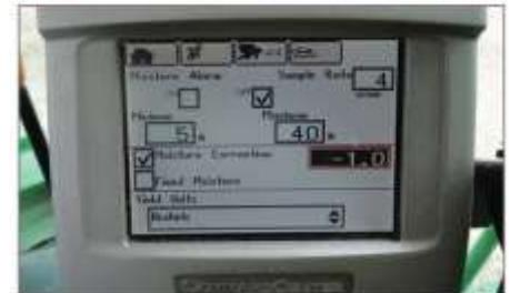
4. Whichever way you need to adjust your number inputted, press the checkmark on the armrest to save your moisture correction value.
