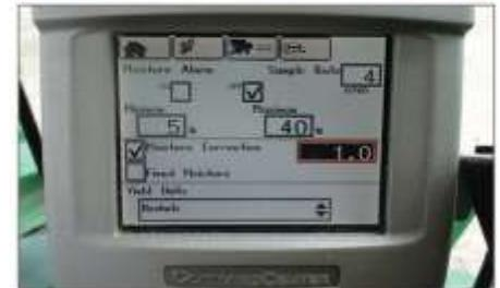
*In this EXAMPLE: Our combine is reading 16% and the coop tested the grain at 15%. We need to subtract 1 from the machine (-1), so we roll the dial to the left.*
