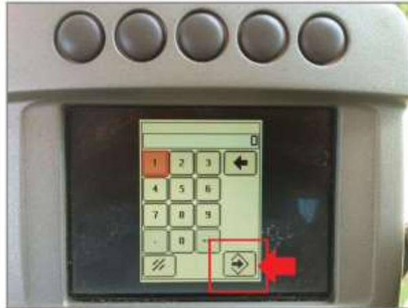
Example: In this example the harvested weight was 3075 lbs. and calibration factor was 652 looking at 2 pictures ago. We inputted 3565 lbs. from the scale and it automatically changed our calibration factor to 562.
