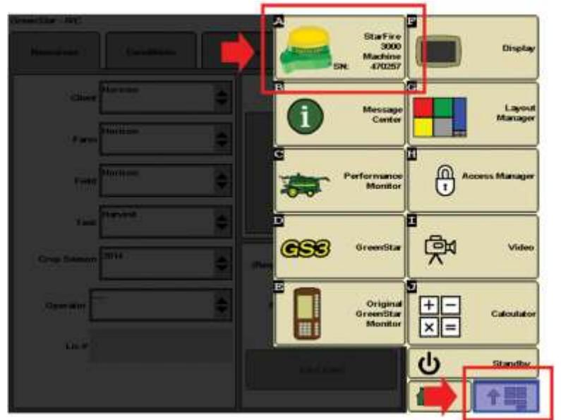
3. Select the G soft key (the tripod with a receiver on it).
