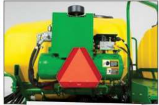
STORAGE TANK & VALVE
