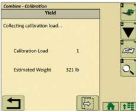
1. Pressing the (return) button will direct the user to the combine calibration selection screen.
