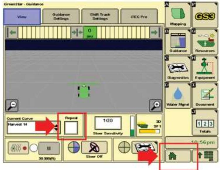
8. Press the "Record" icon. When the record icon is selected, the Red dot next to the icon will start flashing to indicate you are recording your track. Verify the steer icon is on. Drive your first pass. When you turn around, the next pass will appear.
